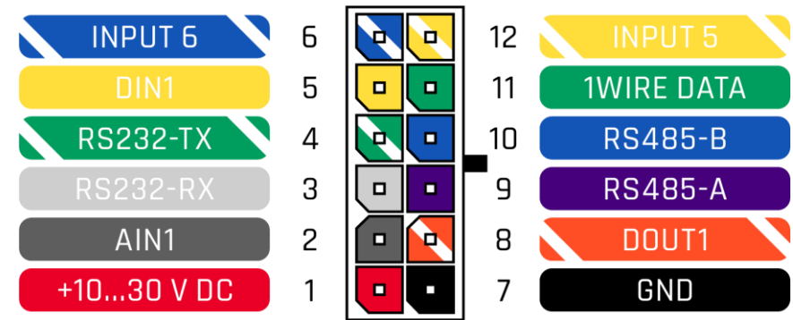
Figure 2 FMC125 2x6 socket pinout
